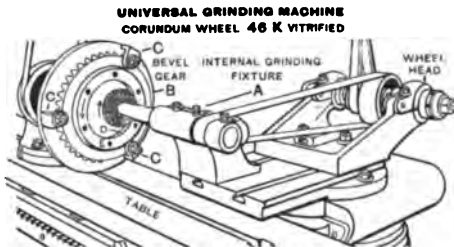
FIG. 22. — GRINDING HOLE IN AUTOMOBILE GEAR.
